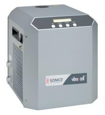
Ultrasonic processing generates heat which may be detrimental to many applications. The chiller automates the cooling process with a 400W cooling capacity and controls temperature from 5-45°C.
