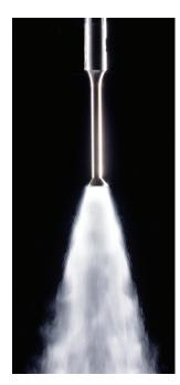
Unlike conventional spray nozzles that rely on high velocity pressure to shear a fluid into small drops, the ultrasonic atomizer uses vibrational energy to generate a low velocity mist. Volumes can vary from microliters to liters, and atomize continuously or intermittently.
