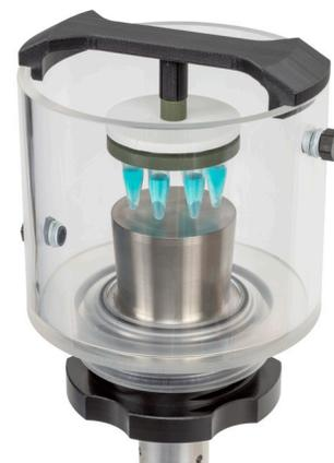
The cup horn is attached to the converter in place of a probe, and filled with water. Microtubes containing samples are placed inside using specially designed tube holders. Ultrasonic energy is transferred through the water and into the sample tubes. Multiple tube holders are available for various size tubes and vessels. Both types of 1.5mL tube holders shown below are included.
