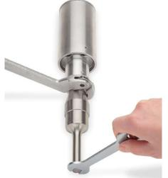
Attach the ½" tip tightly using the wrench set. Once attached the probe is ready to be plugged into the sonicator and tested.
