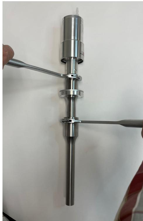
**Note:** parts can be removed by using the wrench set in the opposite manner.
