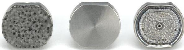
The level of cavitation within a liquid is very much dependent on the surface tension of that liquid and the higher the surface tension the more intense the cavitation. Although water is often chosen as the liquid of choice because it is a great medium for sonic dispersion, consideration should be given to the fact that an ultrasonic probe will typically erode 5 times faster in water than in organic solvents.
