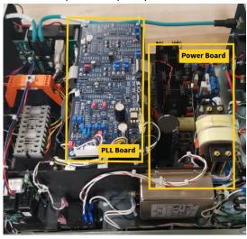
PLL Board: The PLL board is mounted on a bridge frame over top of the Power Board. This board is approximately
