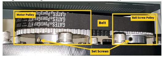
Pulleys: There is a pulley on the motor and on the Ball Screw. These Pulleys transform the rotary motion of the stepper motor to the linear position of the carriage through the Ball Screw.
