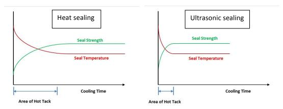
Productivity is further increased with ultrasonic technology because the process does not require any warm up time. The first bag of the day from an ultrasonic VFFS system is perfect. Typical heat seal jaws can require up to 15 minutes of warmup time. 15 minutes @ 80 bags per minute = 1200 additional bags produced using ultrasonics each time the machine is started up.
