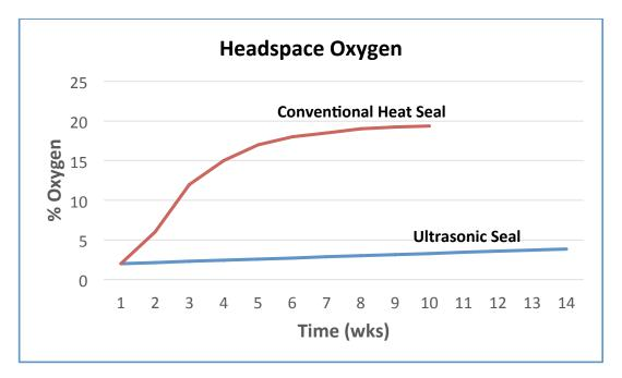
• Further, when ultrasonic technology is used on VFFS baggers, hermetic seals are created even when the film is creased, making the entire process much more forgiving and productive.
