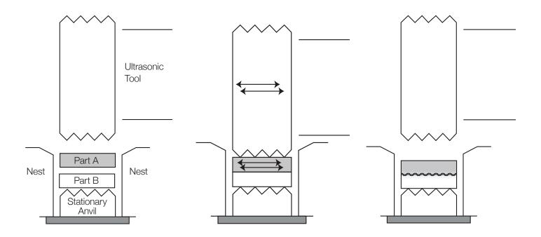
The parts to be welded are placed into a locating nest.
