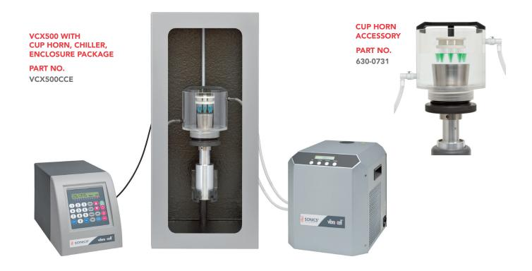
The water-filled cup horn is screwed onto the converter in place of a probe. Microtubes containing the samples are placed inside using specially designed tube holders. Multiple tube holders are available for various size tubes and vessels. Ultrasonic energy is transferred through the water and into the sample tubes.
