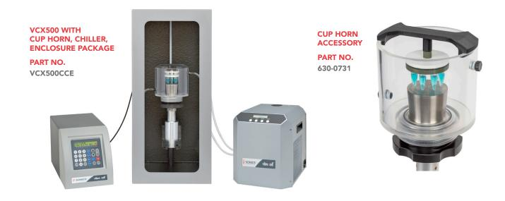
The cup horn is attached to the converter in place of a probe, and filled with water. Microtubes containing samples are placed inside using specially designed tube holders. Ultrasonic energy is transferred through the water and into the sample tubes. Multiple tube holders are available for various size tubes and vessels. Both types of 1.5mL tube holders shown below are included.
