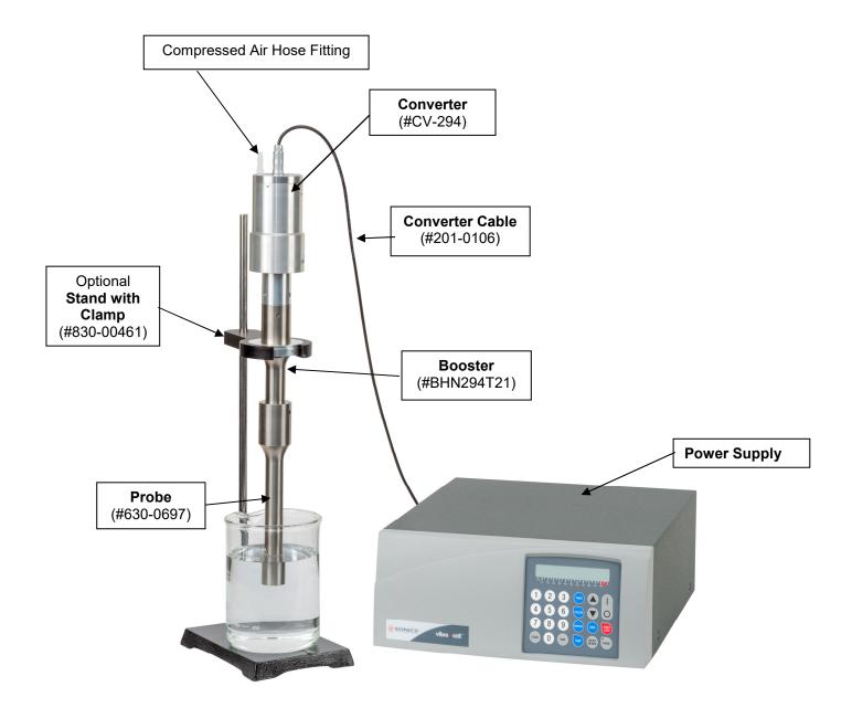
Note: The compressed air hose for cooling the converter is not included.
