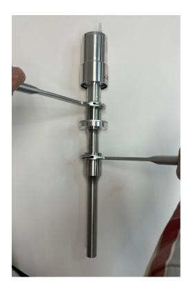
Note: parts can be removed by using the wrench set in the opposite manner.
